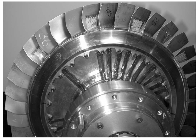
Fig. 6 Blade suction side, 50% span instruments
